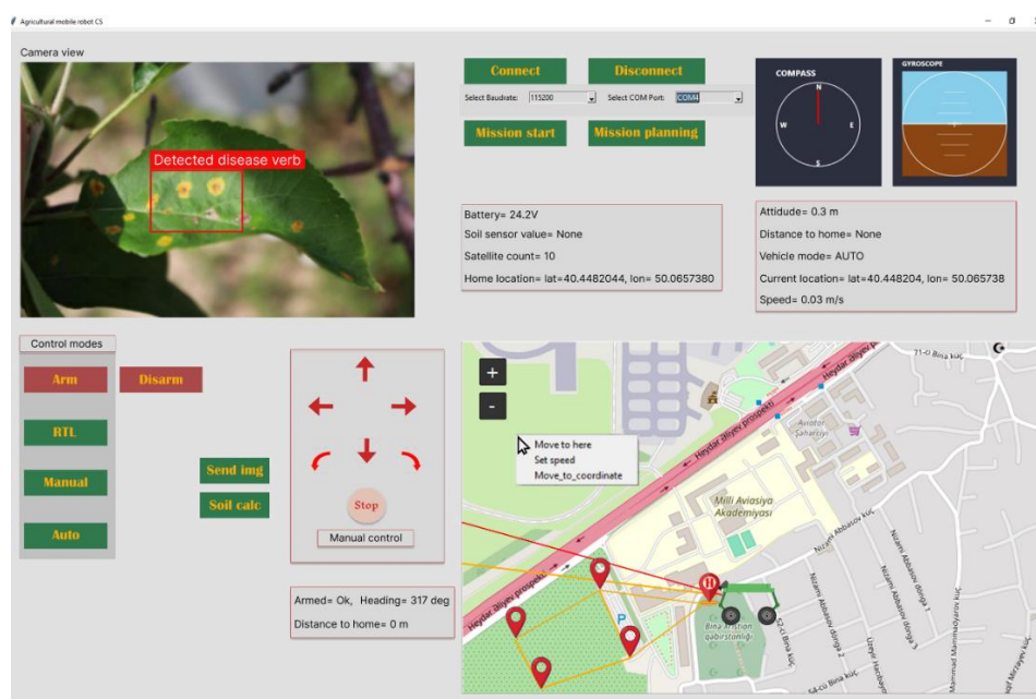
Figure 4. Mission software architecture and real-time sensor visualization interface of the autonomous agricultural rover
